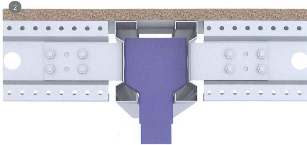
The floor panels transfer the load to the secondary beams, which in turn transfer the load to the main beams ② ③.
